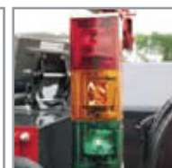
Overload warning lamps + auto stop + alarm
