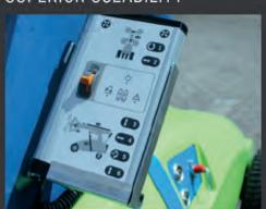
MULTIFUNCTION CONTROL PANEL IN OPERATOR-FRIENDLY DESIGN WITH INTEGRATED BUTTONS AND SIGNAL LIGHTS, DOUBLE ACTION SAFETY KEYS AND GYRO FUNTIONALITY ARE BOTH IN THE STANDARD SETUP ON THE SGL-GR575
